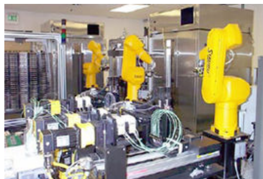
Robots used for the high-throughput screening of chemical libraries to discover new enzyme inhibitors
