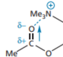
FIGURE 22.16 Neighbouring group participation. The arrow indicates the inductive pull of oxygen which increases the electrophilicity of the carbonyl carbon (see Molecular modelling exercise 22.1).
