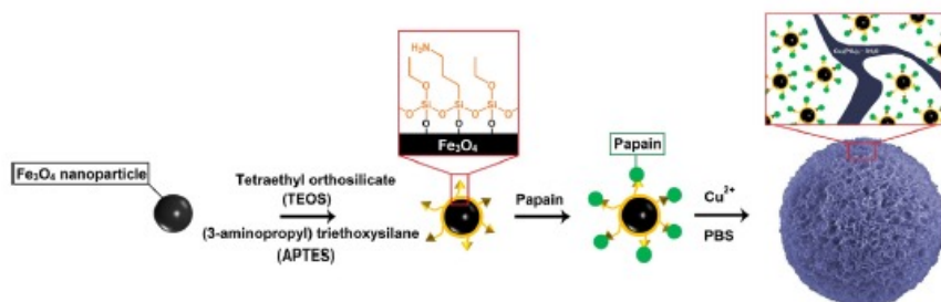
Fig. 1. Schematic diagram of the proposed growth mechanism of PCMN.
