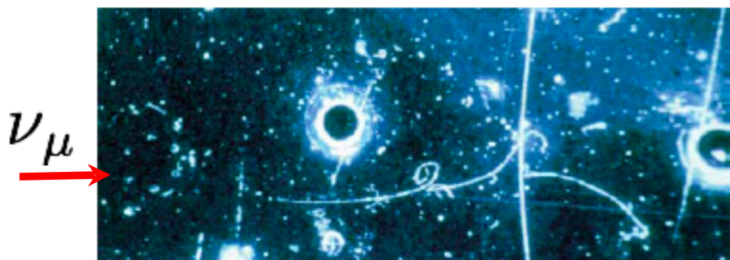
Fig. 1. A hadronic neutral current event, where the interaction of the neutrino from the left produces three secondary particles, all clearly identifiable as hadrons, as they interact with other nuclei in the liquid. There is no charged lepton.
