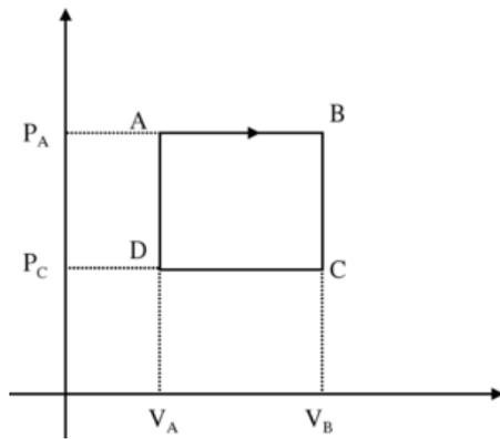
$$p_D = p_C = 2 \text{ atm} \quad p_A = p_B = 4 \text{ atm} \quad V_D = V_A = 20 \text{ l} \quad V_B = V_C = 20 \text{ l}$$
