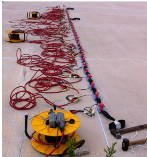
geophones mounted on land streamers
