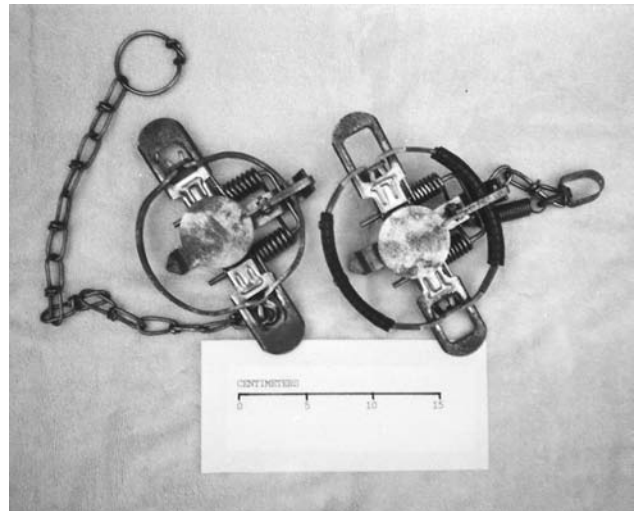
Fig. 3.22. Foothold restraining traps used to capture mammals: Victor No. 1.5 coil spring foothold trap (left) and Victor No. 1.5 Soft-Catch foothold trap with padded jaws (right). Photo by G. F. Hubert, Jr.
