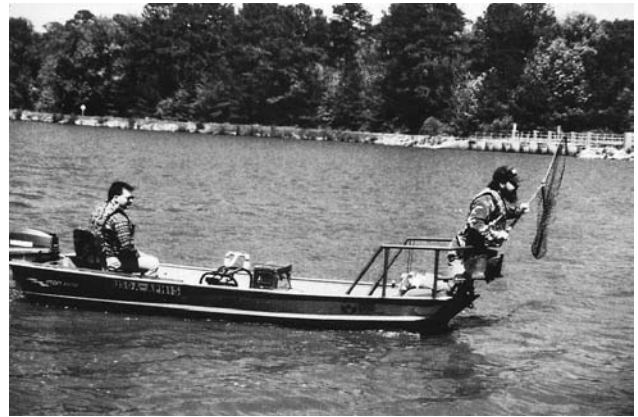
Fig. 3.1. Jon-boat showing positioning of night-lighting equipment (bow rails, lights, converter box, and generator) and personnel. From King et al. (1994).
