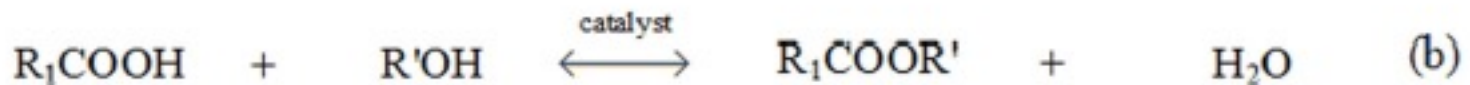
Figure 1. Typical reactions in biodiesel production, (a) transesterification of triglycerides (TG), and (b) esterification of free fatty acids (FFA).
