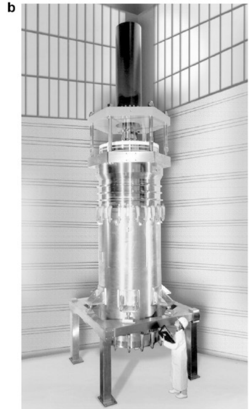
Fig. 1 A generalized overview of the industrial-scale production of modern high-purity recombinant insulins via the “proinsulin route” (a). An industrial-scale preparative HPLC column (photograph courtesy of NovaSep, France) (b)
