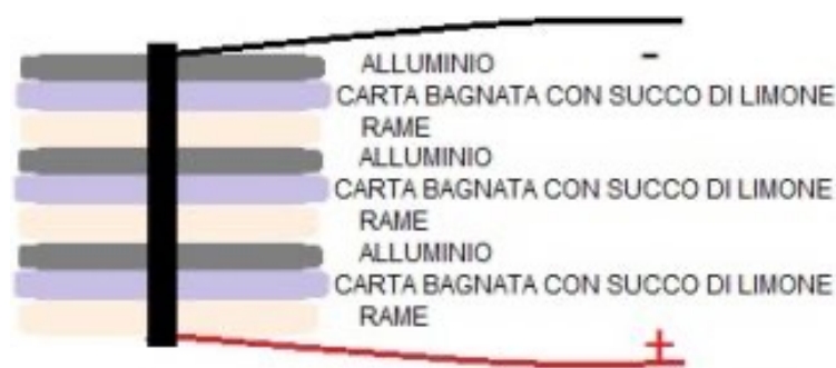
A SIMPLE EXAMPLE OF VOLTAIC PILE
