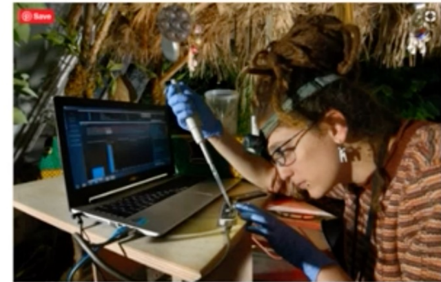
MUSE/Science Museum of Trento The MinION device can sequence small genomes, such as those of bacteria and viruses, displaying the results as they are generated.
