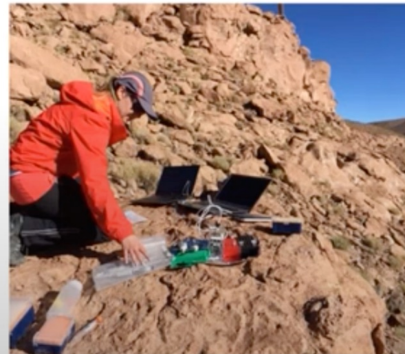
MUSE/Science Museum of Trento The MinION device can sequence small genomes, such as those of bacteria and viruses, displaying the results as they are generated.
