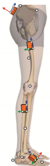
Figure 3. Scheme of the subject instrumented with the MIMUs and the reflective markers. Blue, green and red arrows indicate the X, Y and Z axes of the i th MIMU sensor frame CS_{s_i} .
