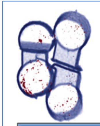
porosity distribution in casted Al specimen
