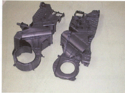
Figure 4.3 Superior and inferior parts of the car evaporator box
