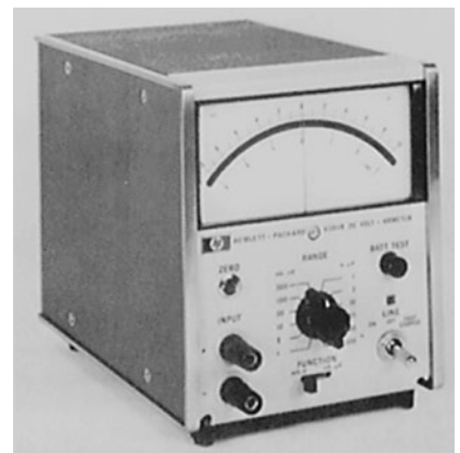
FIGURE 2.15 Electronic-type dc meter with 10-megohm input impedance. (Hewlett-Packard.)
