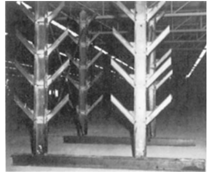
FIGURE 1.3 Plant-made racks for holding steel.
