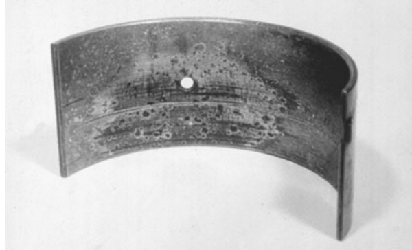
FIGURE 1.8 Bearing with severe dirt embedment.
