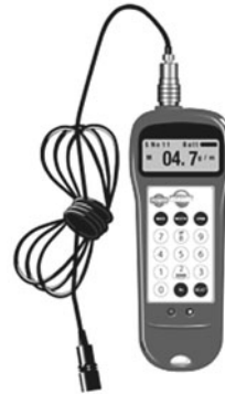
FIGURE 7.22 Sonic tension meter.
