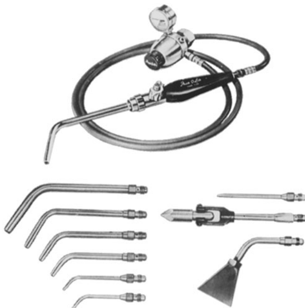
FIGURE 2.1 A typical air-acetylene outfit consisting of a regulator, torch handle, and attached torch stem with interconnecting hose. Also shown are some of the typical interchangeable torch stems available. Notice the special-purpose stems—the hatchet-shaped paint-burner stem and the soldering-iron stem.
