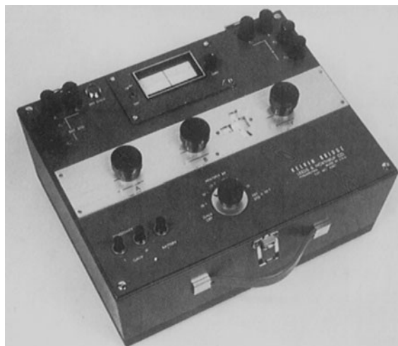
FIGURE 2.29 Portable Kelvin bridge. (Leads and Northrup.)
