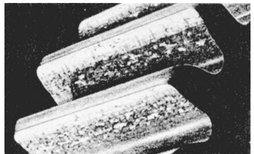
FIGURE 8.5 Severe pitting caused by overloading gear.
