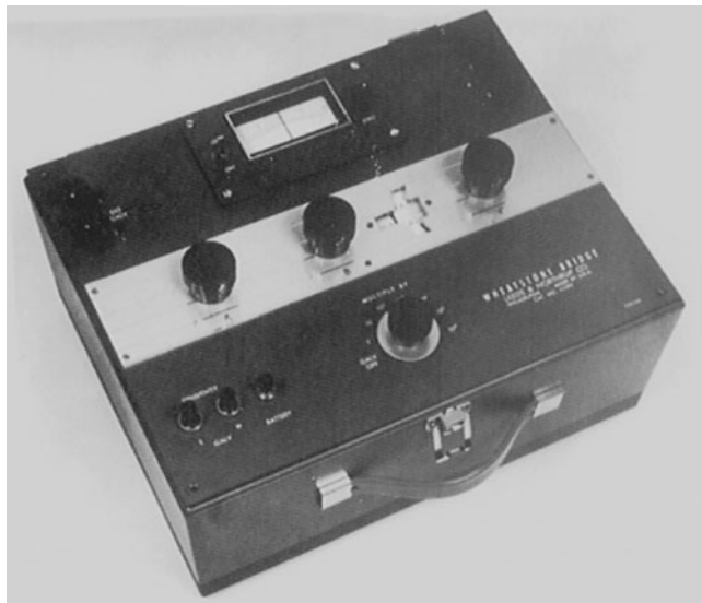
FIGURE 2.27 Portable Wheatstone bridge. (Leeds and Northrup.)
