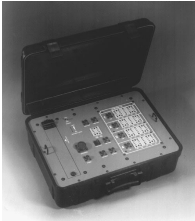
FIGURE 3.2 Jeda jet engine data-acquisition module.
