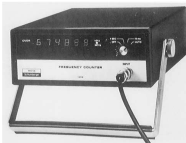
FIGURE 2.31 Portable electronic frequency counter. (Weston Instruments, Inc.)
