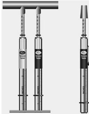
FIGURE 7.21 Pencil-type tension tester.
