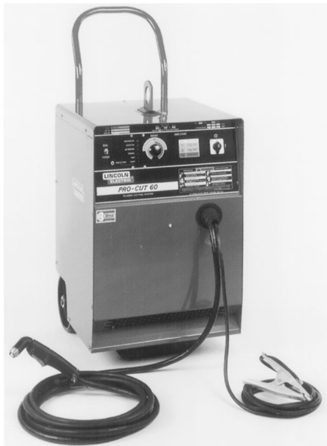
FIGURE 1.30 Power source for plasma arc cutting.
