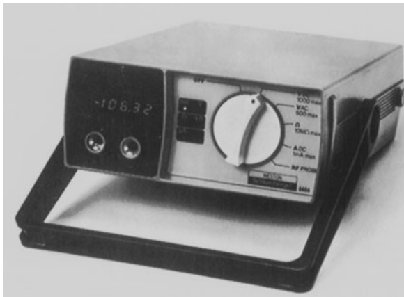
FIGURE 2.6 Four-digit autoranging DMM. (Weston Instruments, Inc.)
