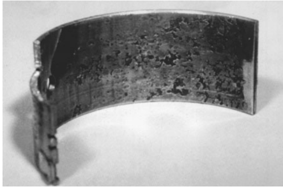
FIGURE 1.10 Fatigue of bearing lining.
