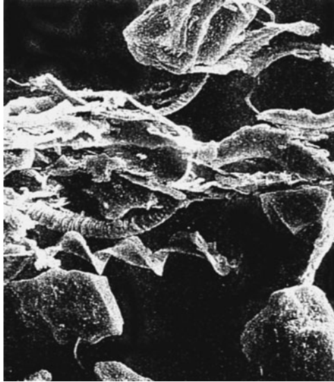
FIGURE 5.3 Typical cutting wear patterns.
