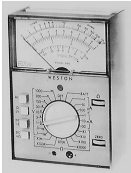
FIGURE 2.3 Typical FET VOM. (Weston Instruments, Inc.)
