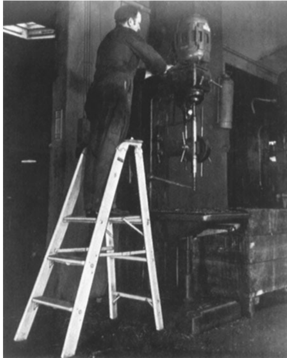
FIGURE 5.2 Platform stepladder. Preferred because it permits worker to have both hands free.
