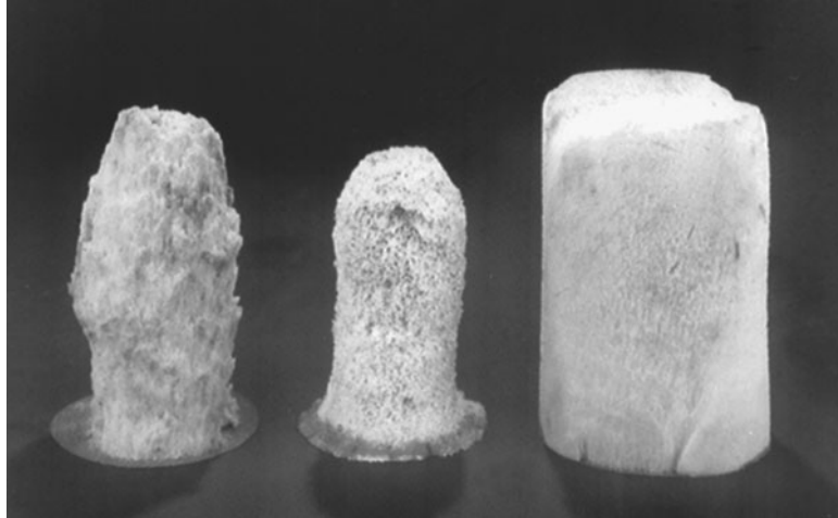
FIGURE 2.5 Pipeline plugs showing deterioration.
