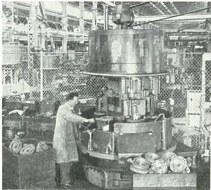
FIG. 118.—Multiple-spindle vertical turret lathe. (Courtesy of The Bullard Company.)
