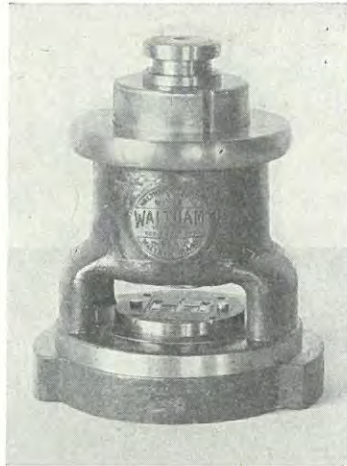
FIG. 15.—A self-contained subpress die. (Courtesy of the Waltham Machine Works.)
