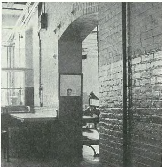
FIG. 87.—Blind corner mirror. (Courtesy of the National Conservation Bureau.)
