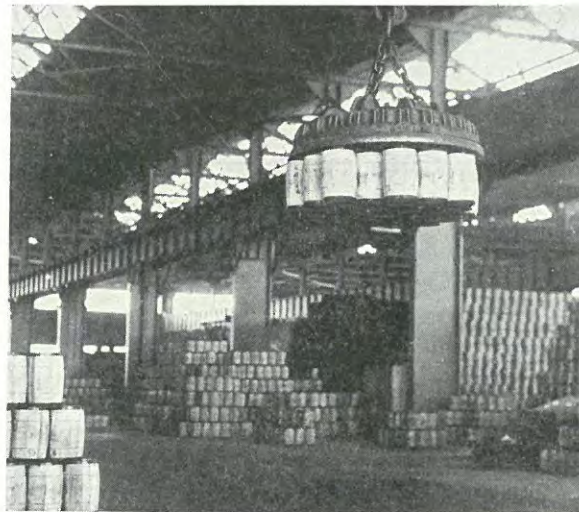
FIG. 48.—Handling materials with an electromagnet. (Courtesy of the Electric Controller & Manufacturing Company.)
