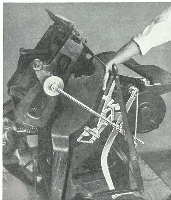
FIG. 55.—Job-printing-press platen guard. (Courtesy, The Travelers Insurance Co.)
