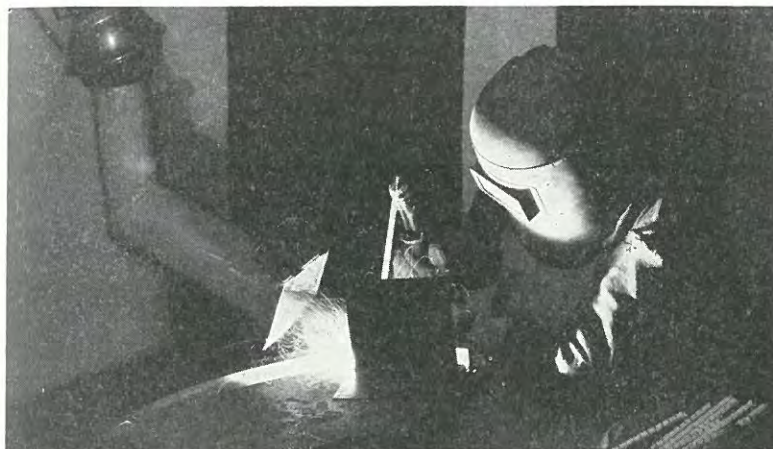
FIG. 136.—Turbine diaphragm being arc-welded. (Courtesy of the General Electric Company.)
