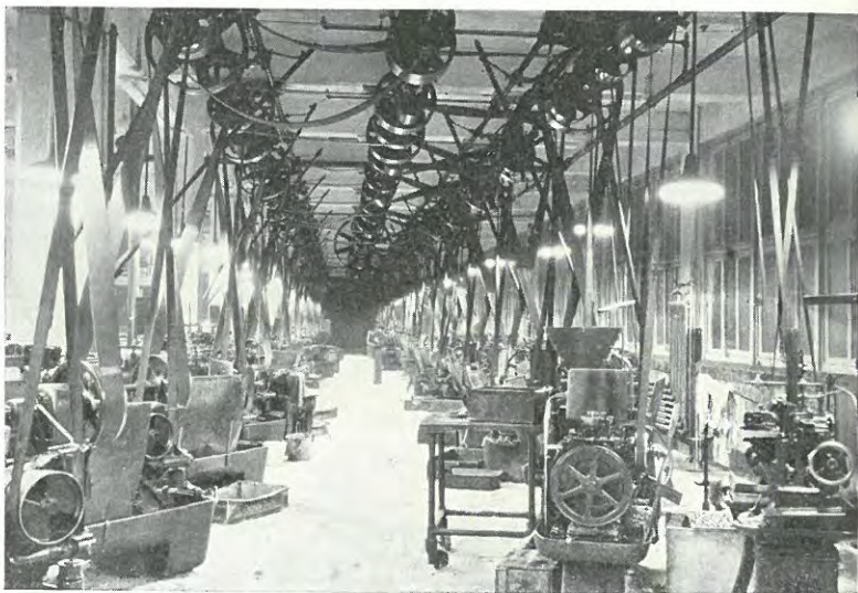
FIG. 130.—A veritable maze of transmission belts and pulleys, also machine belts, pulleys, and moving parts. (Courtesy of the National Conservation Bureau.)
