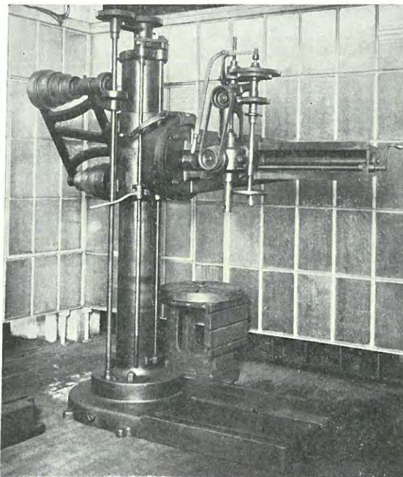
FIG. 96.—Radial drill with unguarded machine hazards. (Courtesy of The Cincinnati Bickford Tool Company.)
