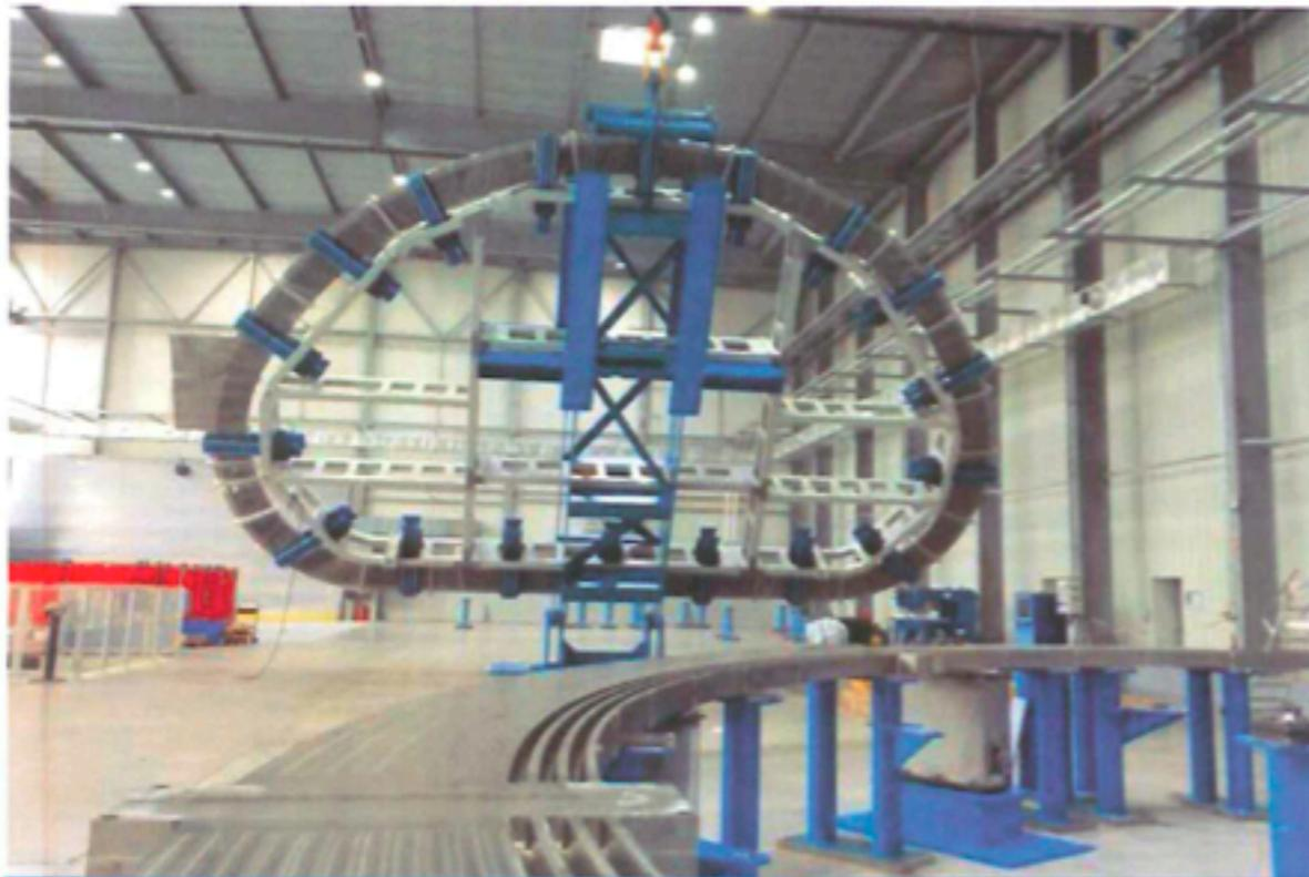
Radial Plates being manufactured at SIMIC
