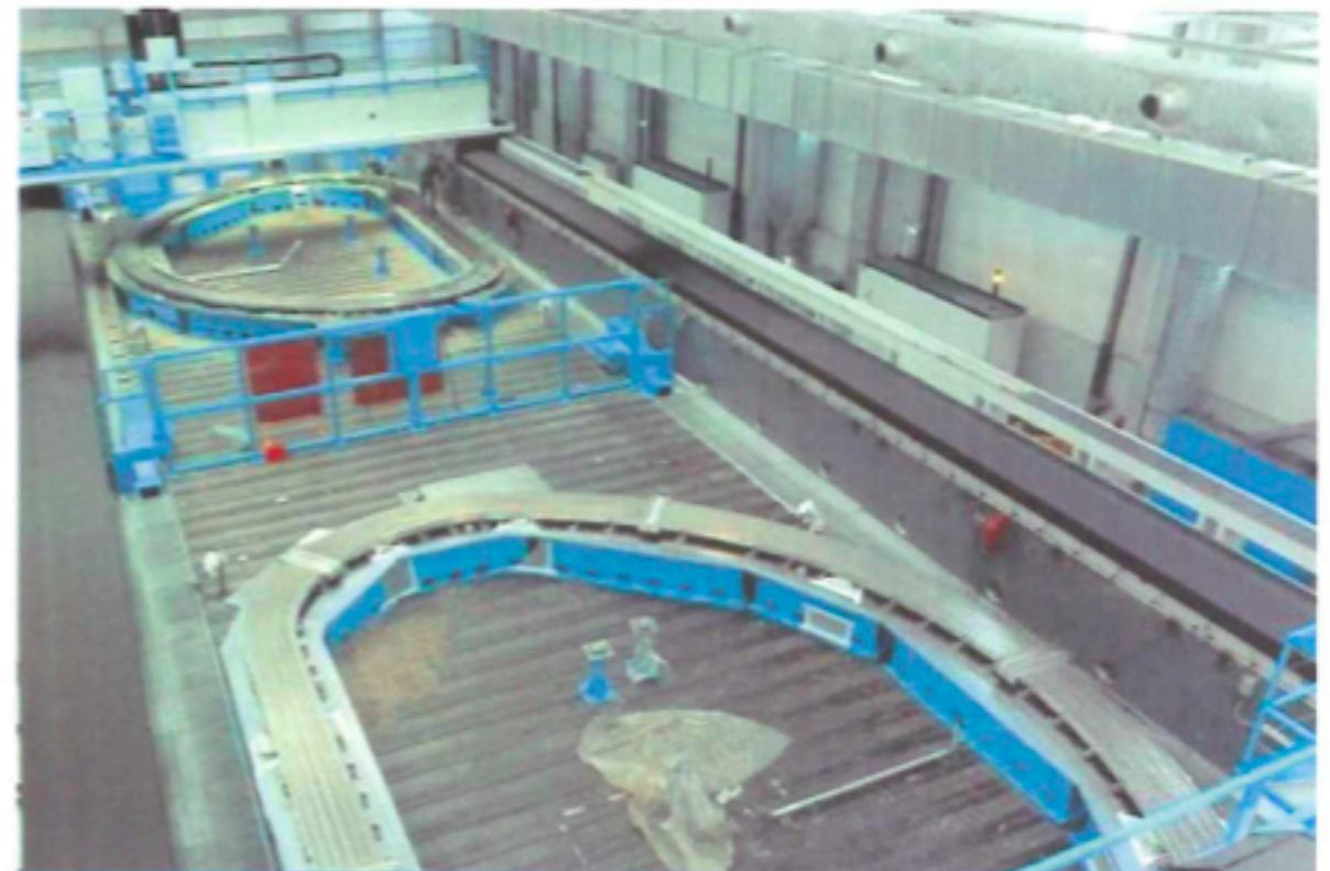
Radial Plates being manufactured at CNIM
