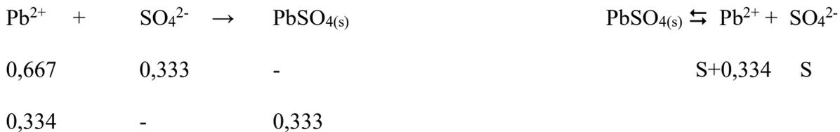
$$E = E^\circ + \frac{0.0592}{2} \log[Pb^{2+}] = -0,13 + \frac{0.0592}{2} \log[0,334] = -0,144 \text{ V}$$
