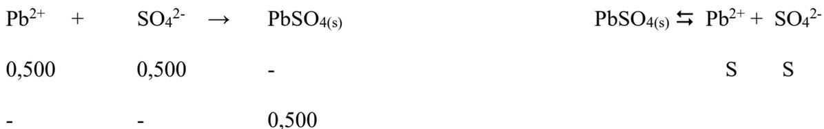
$$E = E^\circ + \frac{0.0592}{2} \log[Pb^{2+}] = -0,13 + \frac{0.0592}{2} \log K_s^{0,5} = -0,248 \text{ V}$$
