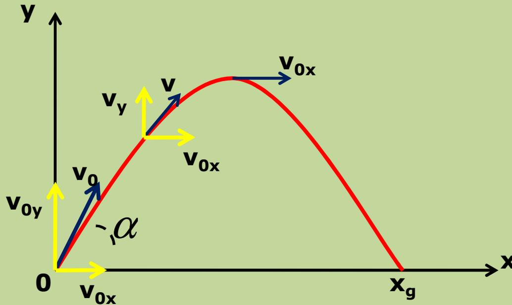
$$v_{0x} = v_0 \cos \alpha$$
