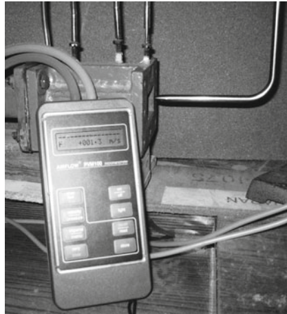
Fig. 8.3 Photograph of a Pitot tube with a digital micro-manometer that displays velocity directly
