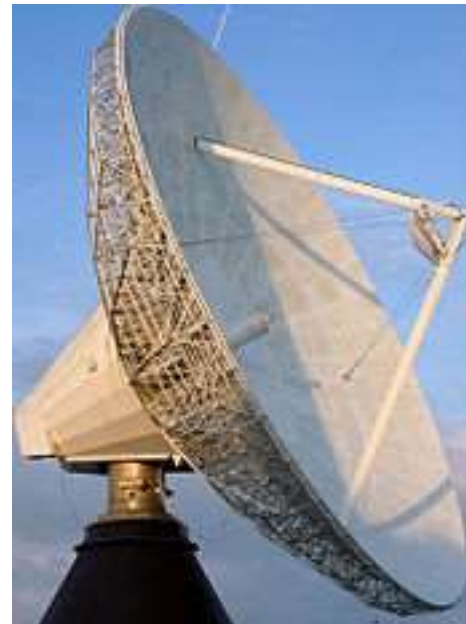
Cassegrain configuration: parabolic reflector, hyperbolic sub-reflector
