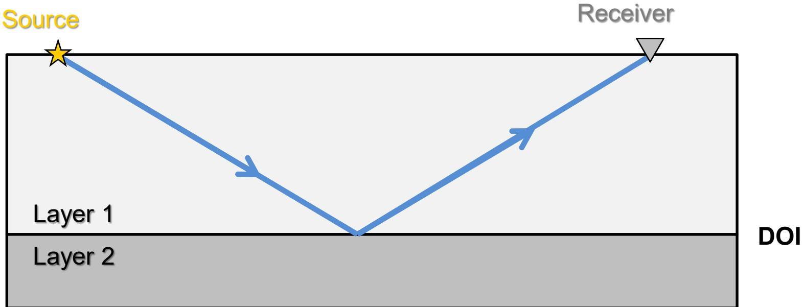
Depth of investigation depends on the wavelength of the signal. The higher is the wavelength the lower will be the depth of investigation
