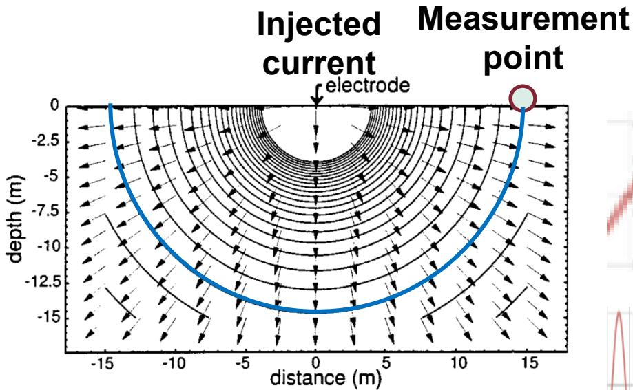
Resolution rapidly decreases with depth proportionally to the spacing of equipotential lines
