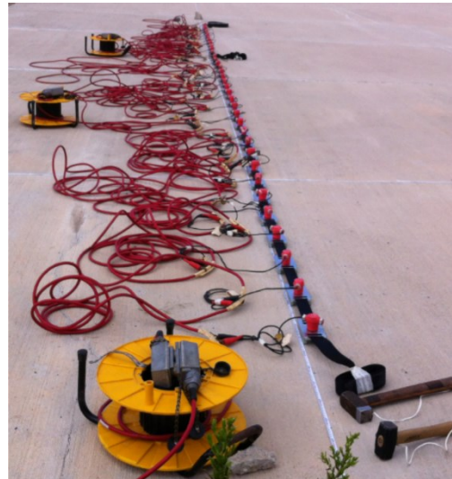
geophones mounted on land streamers
