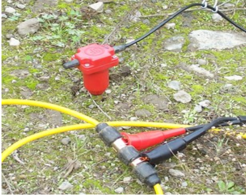
Vertical 10 Hz- geophone with cable connections
