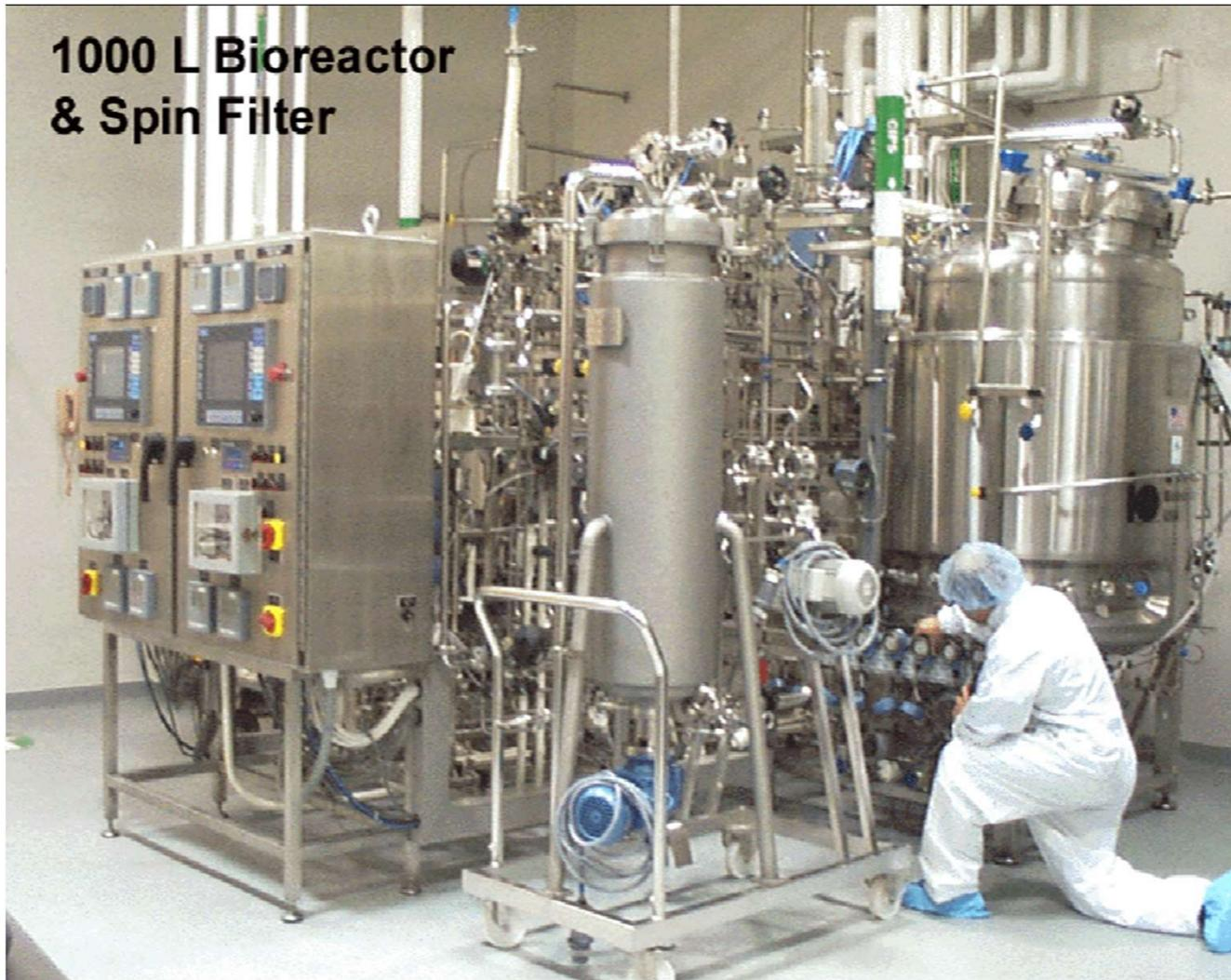
Example of a 1000 L Bioreactor with an external spin filter used in the production of Remicade® in Malvern, PA
