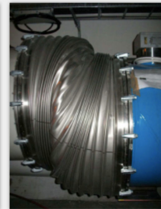
2 most severely damaged interconnects
