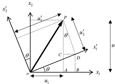
**Figure 7.1.3: geometry of the 2D coordinate transformation**
