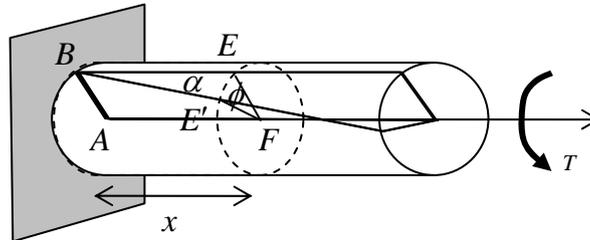
**Figure 7.2.2: A section of a twisting cylindrical member**
