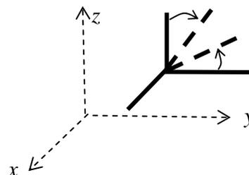
**Figure 4.1.17: strains occurring in the  $y-z$  plane**
