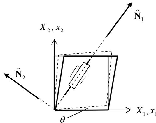
Figure 2.2.12: simple shear
