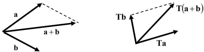
Figure 1.8.1: Linearity of the second order tensor
