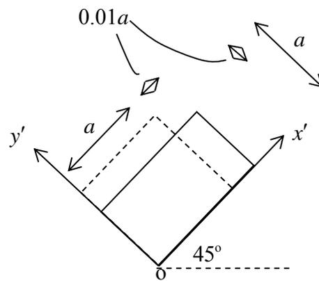
**Figure 4.2.5: Principal strains for the block in pure shear**
