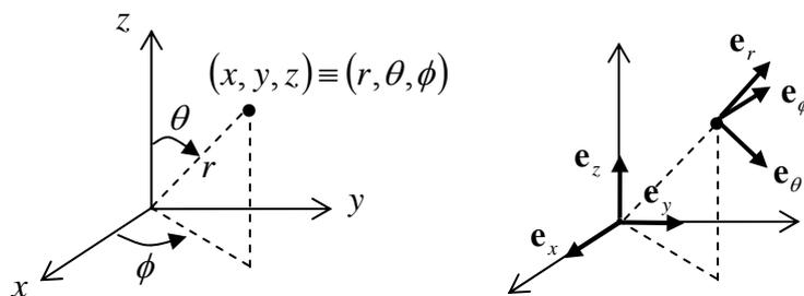
**Figure 1.6.9: spherical coordinates**
