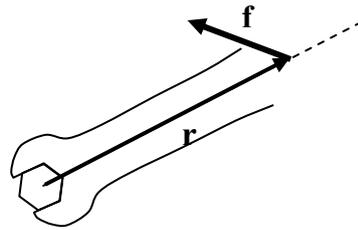
Figure 1.8.3: the force on a spanner
