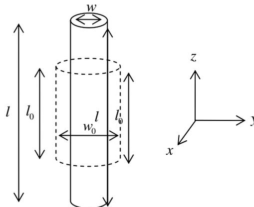
**Figure 5.2.5: Change in dimensions of a test specimen**
