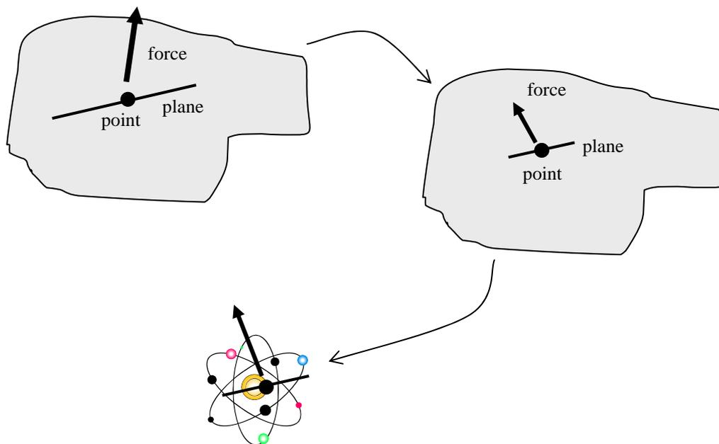
**Figure 5.4.1: A force acting on an internal surface; allowing the plane on which the force acts to get progressively smaller**
