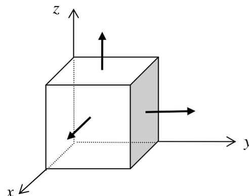
8. By the definition of the traction vector  $\mathbf{t}$  which acts on the  $x-z$  plane,  $\mathbf{t}^{(i)} = \sigma_{yx}\mathbf{i} + \sigma_{yy}\mathbf{j} + \sigma_{yz}\mathbf{k}$ . Sketch these three stress components on the figure below.
