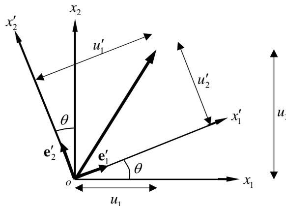
**Figure 1.5.2: a vector represented using two different coordinate systems**
