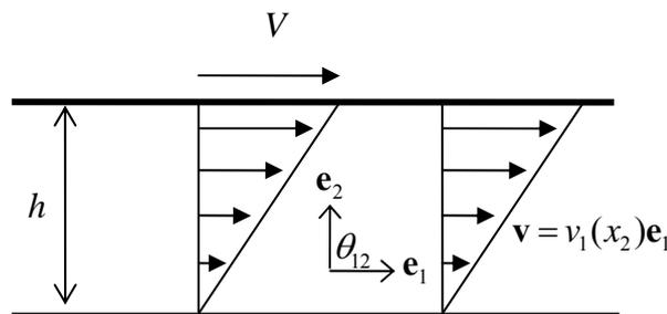
Figure 2.5.2: shear flow
