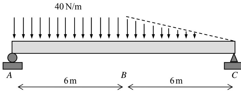
**Figure 7.4.13: a beam subjected to a distributed load**
