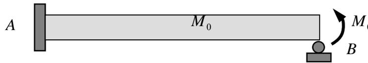
Figure 7.4.36: a statically indeterminate beam
