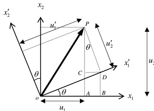
**Figure 1.5.3: geometry of the 2D coordinate transformation**
