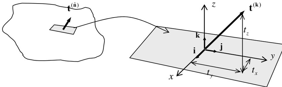
**Figure 3.3.7: the components of the traction vector**
