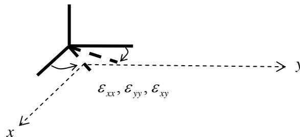
**Figure 4.2.1: non-zero strain components acting in the  $x - y$  plane**
