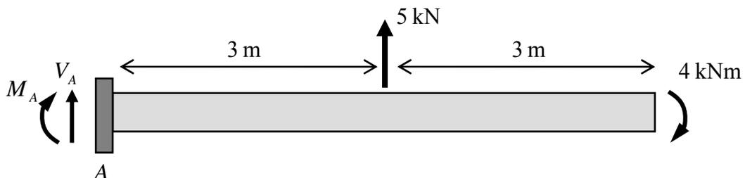
**Figure 7.4.10: a cantilevered beam loaded by a force and moment**
