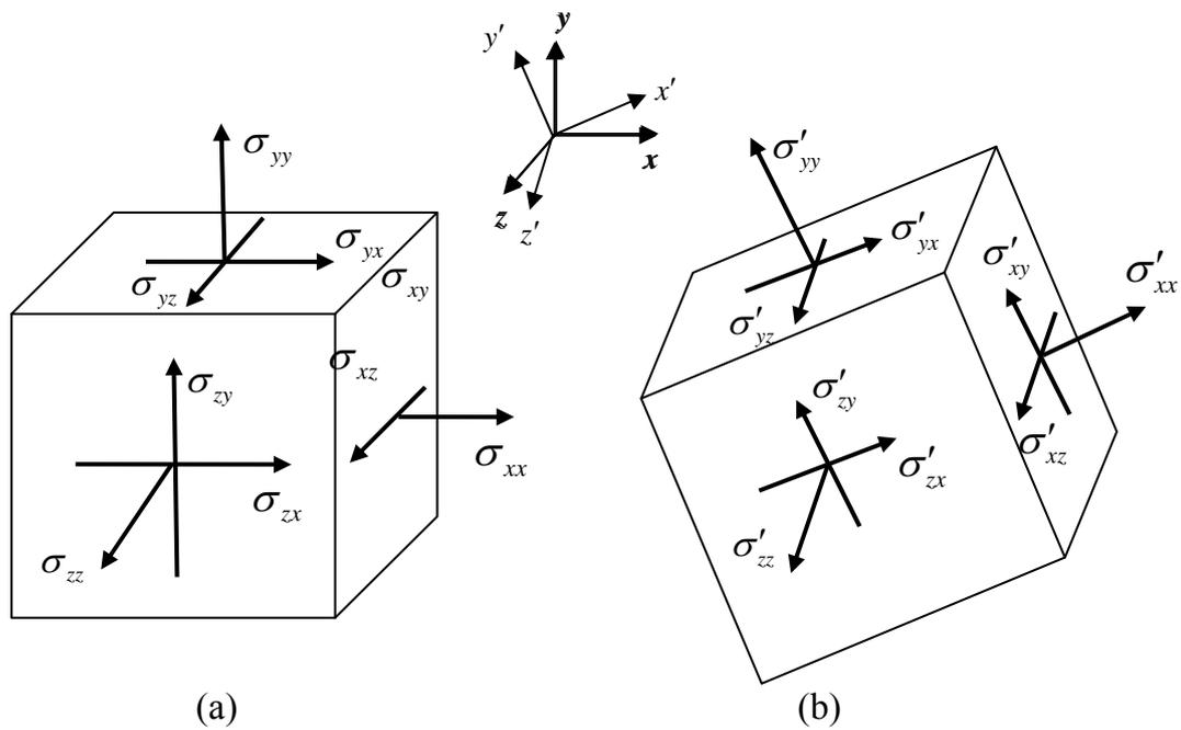
**Figure 3.4.5: a three dimensional material element; (a) original element, (b) rotated element**
