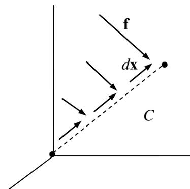
Figure 1.7.1: a particle moving in a force field
