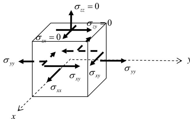
**Figure 3.5.6: stresses acting on the  $x - y$  plane**
