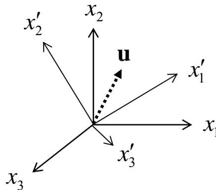
**Figure 1.5.4: two different coordinate systems in a 3D space**
