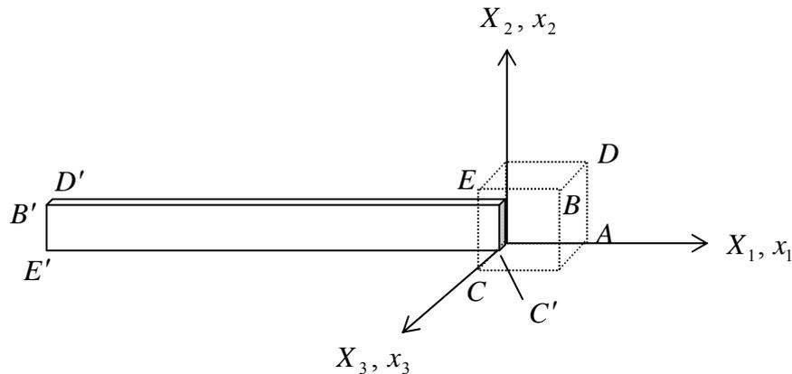
Figure 2.2.3: a deforming cube
