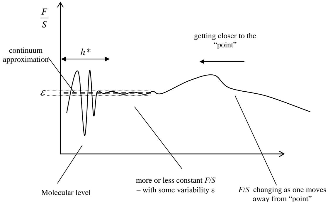
**Figure 5.4.2: the change in traction as the plane upon which a force acts is reduced in size**
