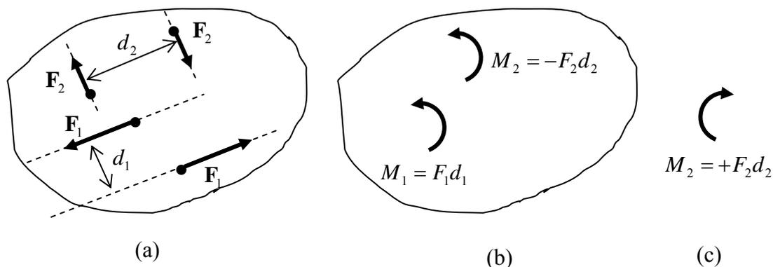
**Figure 2.3.4: Two couples acting on a rigid body**
