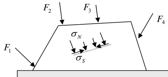
**Figure 3.3.3: a component subjected to a complex loading, giving rise to a non-uniform stress distribution over an internal surface**
