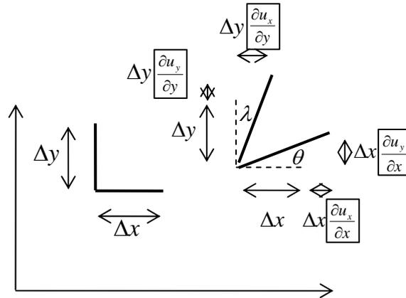
Figure 1.2.4: strains in terms of displacement gradients
