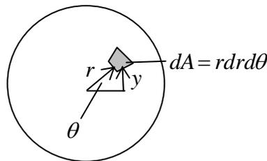
**Figure 7.2.23: Moment of inertia for a circular cross-section**
