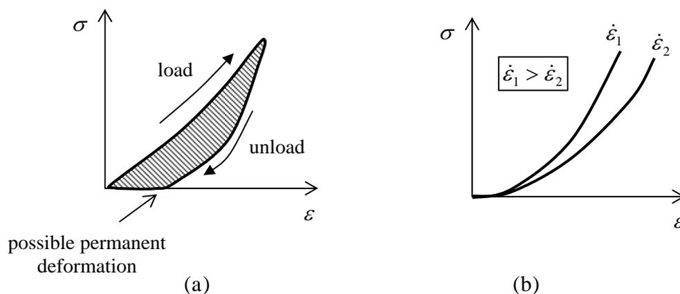
**Figure 5.3.2: Response of a Viscoelastic material in the Tension test; (a) loading and unloading with possible permanent deformation (non-zero strain at zero stress), (b) different rates of stretching**
