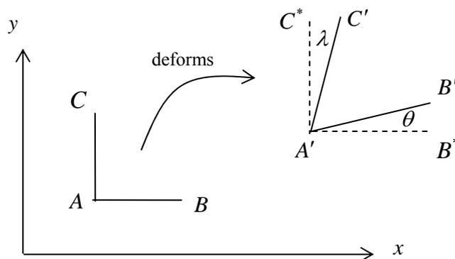
**Figure 4.1.10: small deformation**
