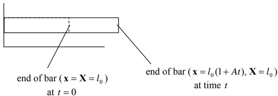
**Figure 3.1.6: a stretching bar**
