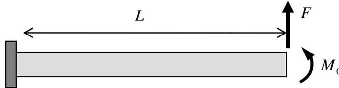
**Figure 7.4.31: a cantilevered beam loaded by an end-force and moment**
