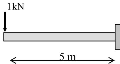
5. Consider the cantilever beam shown below. Determine the maximum shearing stress in the beam and determine the shearing stress 25 mm from the top surface of the beam at a section adjacent to the supporting wall. The cross-section is the “T” shape shown, for which  $I = 40 \times 10^6 \text{ mm}^4$ .
