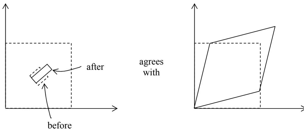
**Figure 4.2.6: Strain viewed from two different coordinate systems**
