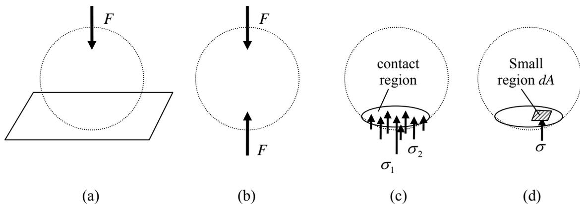
**Figure 3.1.2: a ball being forced into a large object, (a) force applied to ball, (b) reaction of object on ball, (c) a non-uniform stress distribution over the contacting surface, (d) the stress acting on a small (infinitesimal) area**
