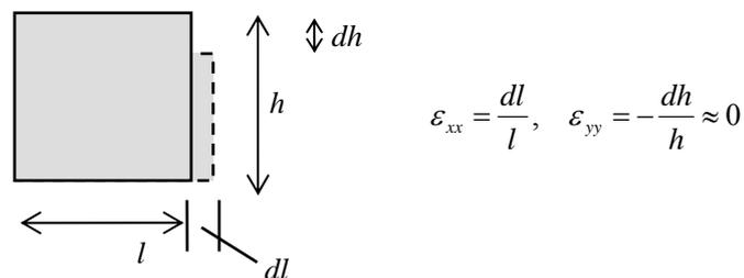
**Figure 7.4.20: transverse strain is neglected in the elementary beam theory**
