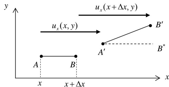
**Figure 1.2.1: deformation of a line element**
