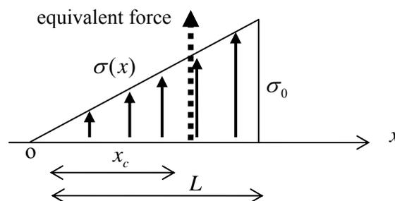
**Figure 3.1.4: triangular stress distribution and equivalent force**
