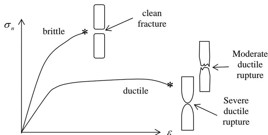
**Figure 5.2.8: the difference between ductile and brittle materials**
