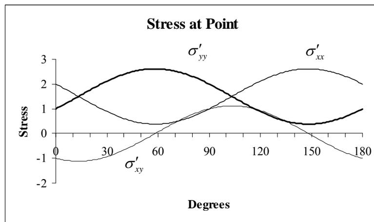
**Figure 3.5.3: stresses on different planes through a point**
