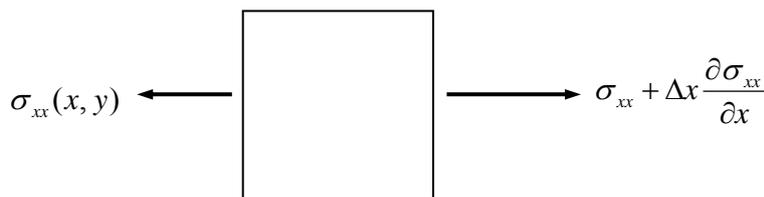
**Figure 1.1.5: net stresses acting on a differential element**
