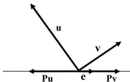
**Figure 1.8.5: the projection tensor**
