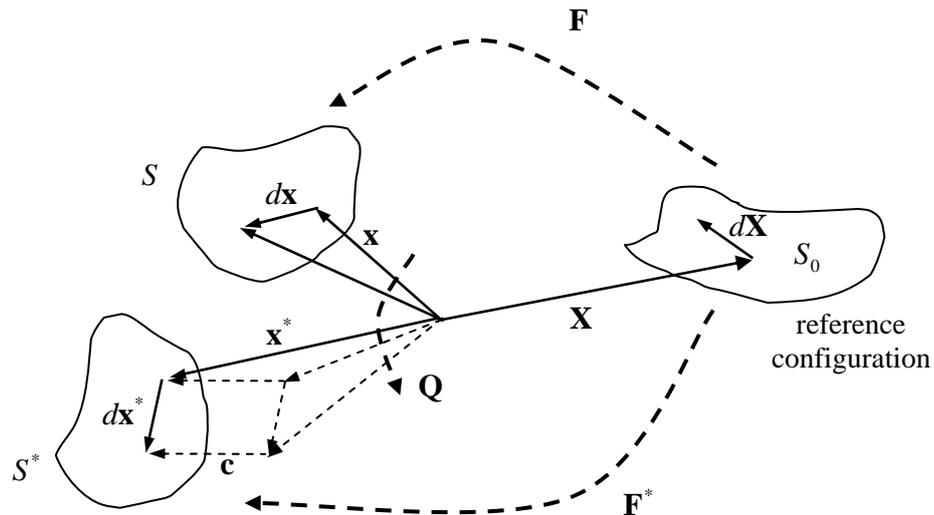
**Figure 2.9.1: a rigid body rotation and translation of the current configuration**
