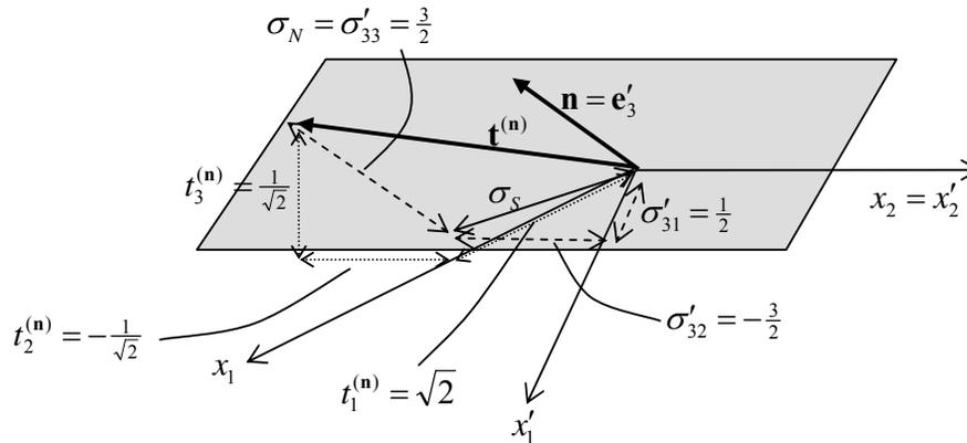
Figure 7.2.9: traction and stresses acting on a plane
