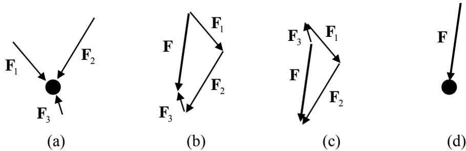
**Figure 2.1.2: the resultant of a system of forces acting on a particle; (a) three forces acting on a particle, (b) construction of the resultant  $\mathbf{F}$ , (c) an alternative construction, showing that the order in which the forces are drawn is immaterial, (d) the resultant force acting on the particle**
