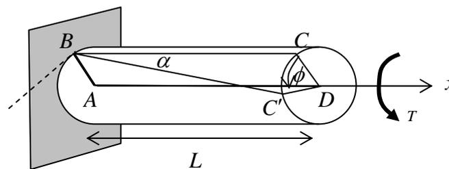
**Figure 7.2.1: A cylindrical member under the action of a torque**
