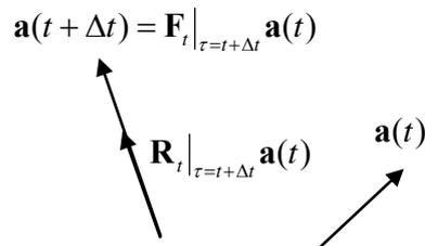
Figure 2.6.1: rotation and stretch of a vector
