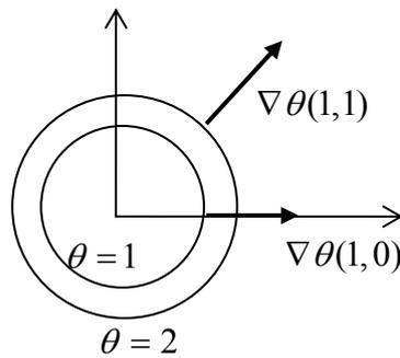
**Figure 1.6.5: gradient of a temperature field**
