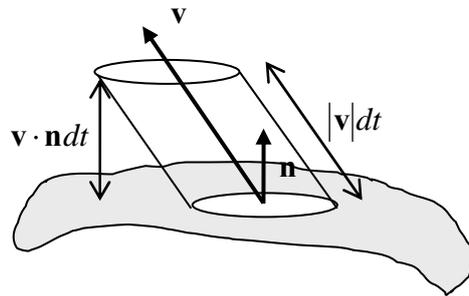
**Figure 1.7.7: flow through a surface element**
