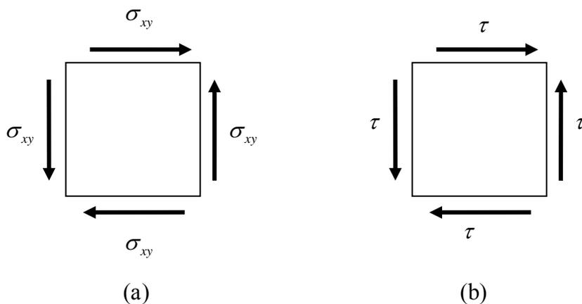
**Figure 3.4.3: shear stress acting on a material element**
