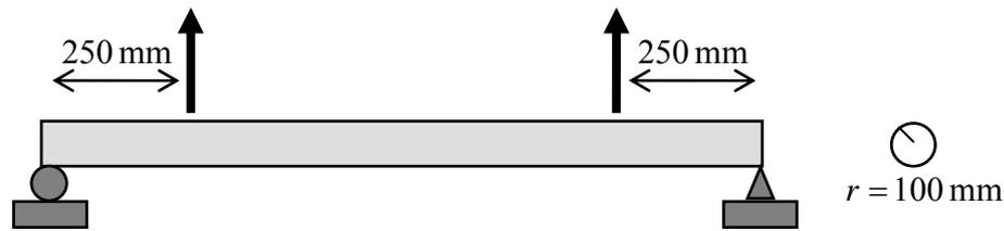
**Figure 7.4.24: a loaded beam with circular cross-section**
