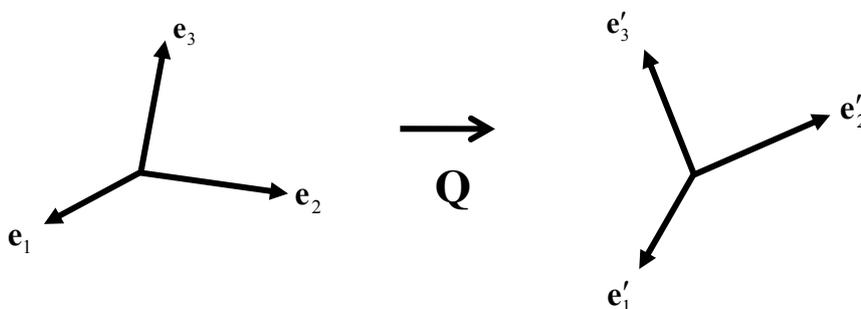
Figure 1.10.2: Rotation of a set of base vectors
