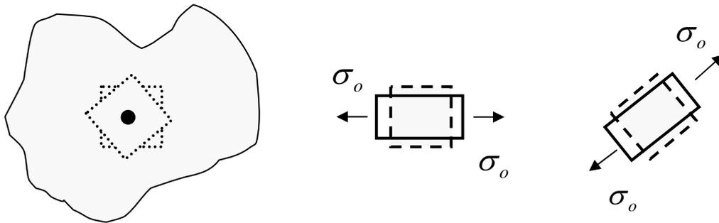
**Figure 5.2.17: Illustration of Isotropy; the stress-strain response is the same no matter in what “direction” the test specimen is cut from the material**
