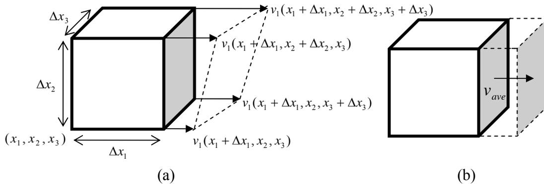
**Figure 1.6.6: a differential element; (a) flow through a face, (b) volume of material flowing through the face**
