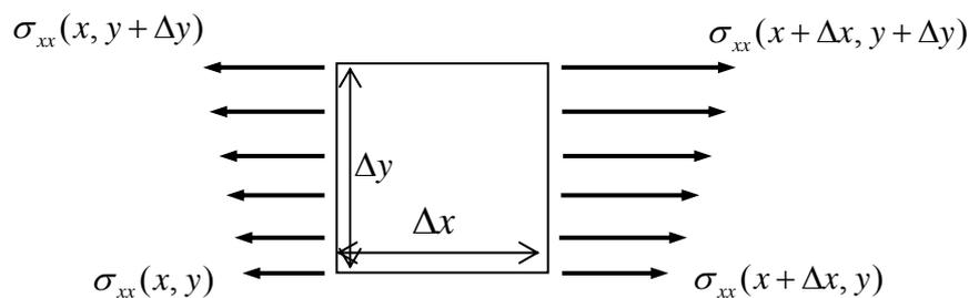
**Figure 1.1.3: varying stresses acting on a differential element**
