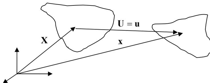
Figure 2.2.13: the displacement
