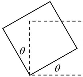
**Figure 4.1.15: an element undergoing a rigid body rotation**
