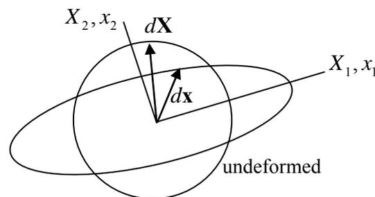
**Figure 2.2.9: a circular element deforming into an ellipse**
