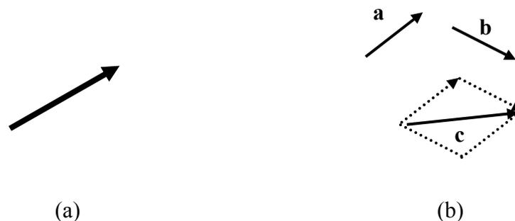
Figure 1.1.1: (a) a vector; (b) addition of vectors
