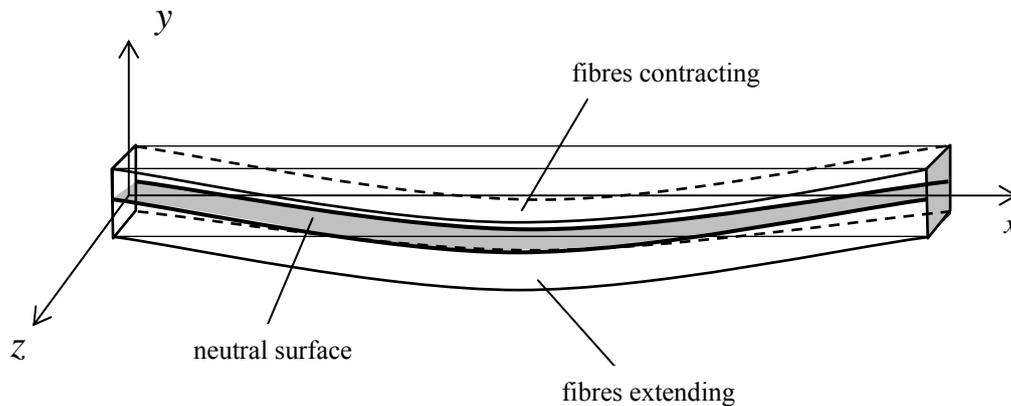
**Figure 7.4.3: the neutral surface of a beam**
