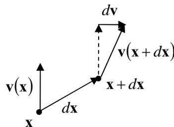
**Figure 2.5.1: velocity gradient**
