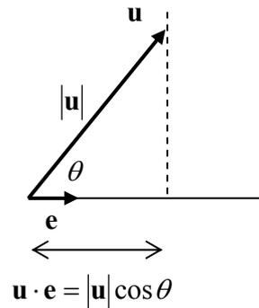
**Figure 1.1.5: the projection of a vector along the direction of a unit vector**
