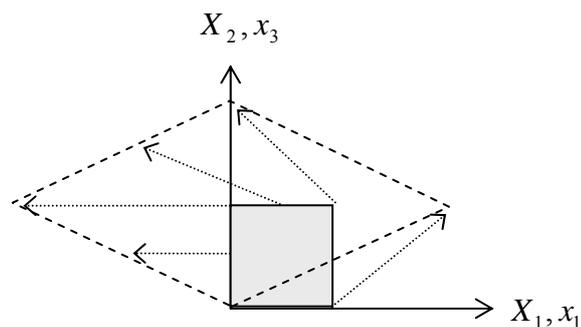
**Figure 2.2.5: deformation of a square**
