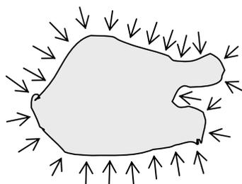
**Figure 3.5.12: a material subjected to atmospheric pressure**
