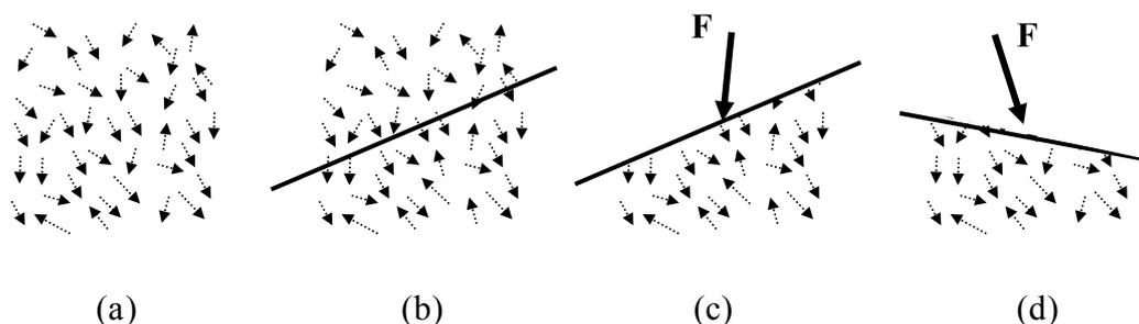
**Figure 3.3.4: a multitude of molecular forces represented by a single force; (a) molecular forces, a plane drawn through the material, replacing the molecular forces with an equivalent force  $\mathbf{F}$ , a different equivalent force  $\mathbf{F}$  acts on a different plane through the same material**
