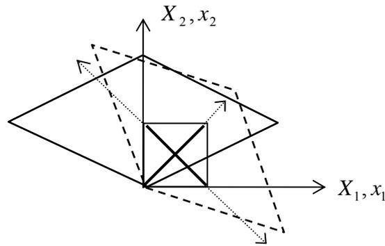
Figure 2.2.7: stretch and rotation of a square
