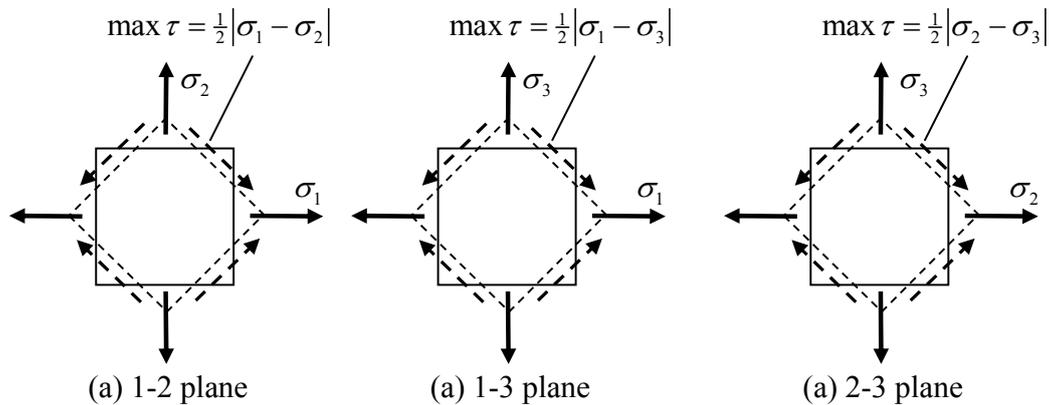
**Figure 3.5.8: principal stresses and maximum shear stresses**
