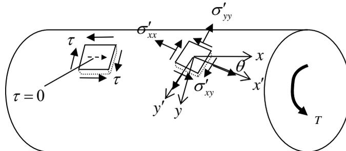
**Figure 7.2.6: Stress distribution in a torsion member**
