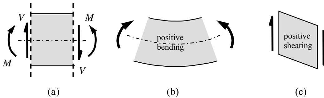
**Figure 7.4.5: sign convention for moments and shear forces**
