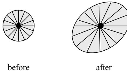
**Figure 2.2.2: deformation of a material particle**
