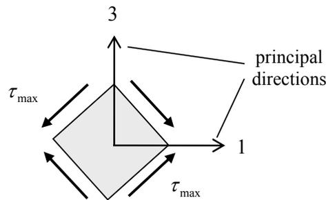
**Figure 7.2.14: maximum shear stress at a point**
