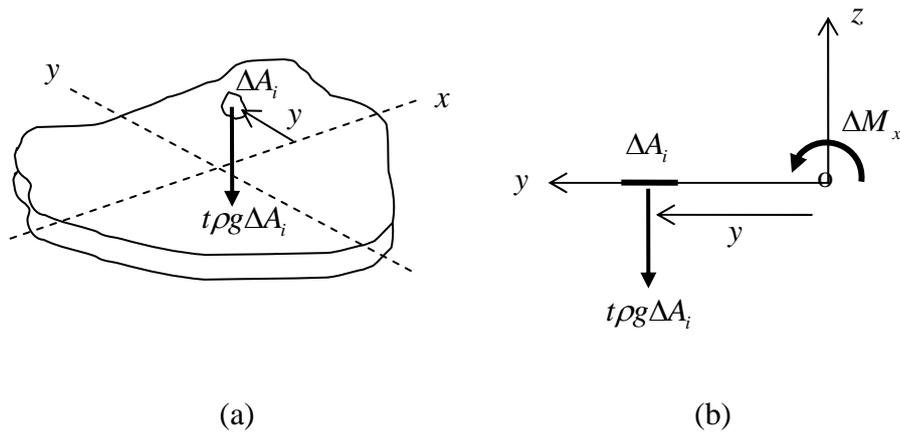
**Figure 3.2.3: The moment  $M_x$ ; (a) full view, (b) plane view**
