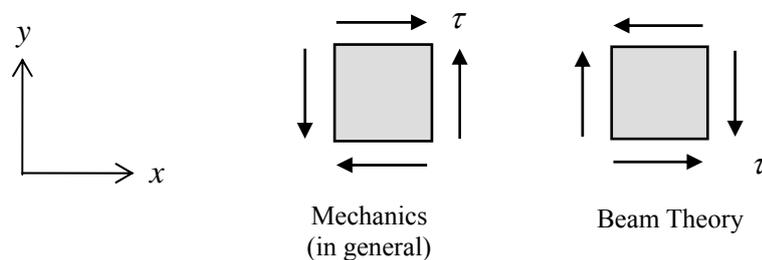
**Figure 7.4.6: sign convention for shear stress in beam theory**
