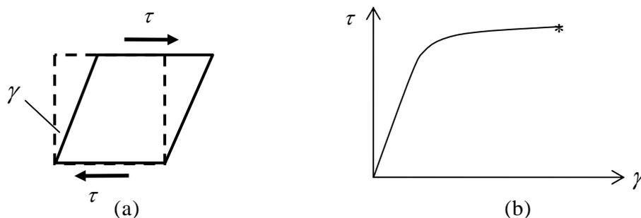
**Figure 5.2.11: the shear test; (a) specimen subjected to shear stress and shear strain (dotted = undeformed), (b) shear stress-strain curve**
