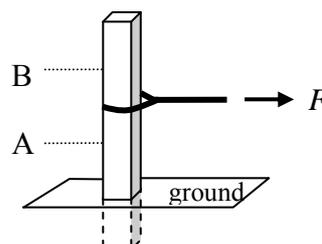
4. In Fig. 3.3.11, which of the stress components is/are negative?
