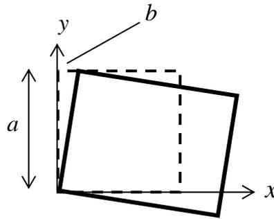
**Figure 1.2.8: an element undergoing a normal strain and a rotation**
