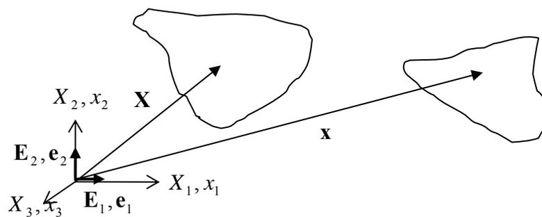
**Figure 2.1.4: reference and current configurations with coincident axes**
