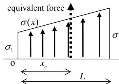
**Figure 3.1.5: a non-uniform stress distribution and equivalent force**
