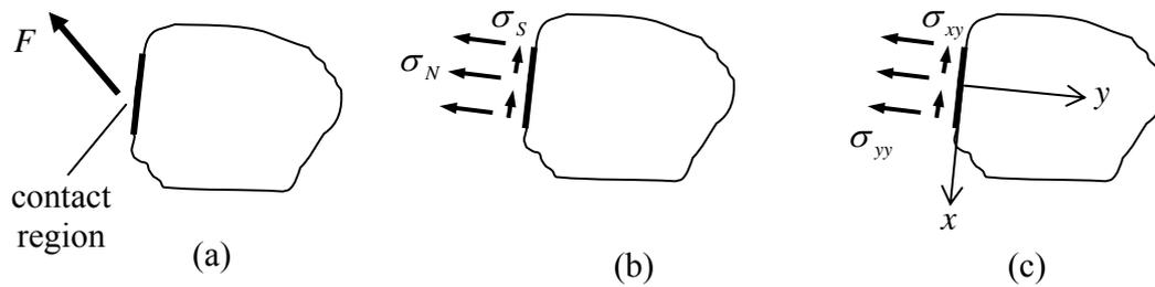
**Figure 3.5.9: Stress boundary conditions; (a) force acting on material due to contact with a second material, (b) the resulting normal and shear stress distributions, (c) applied stresses as stress components in a given coordinate system**
