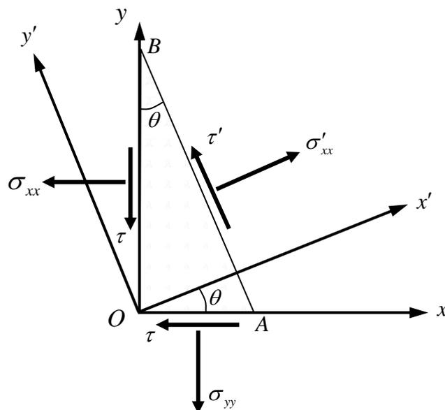
**Figure 3.4.7: a free body diagram of a triangular element of material**
