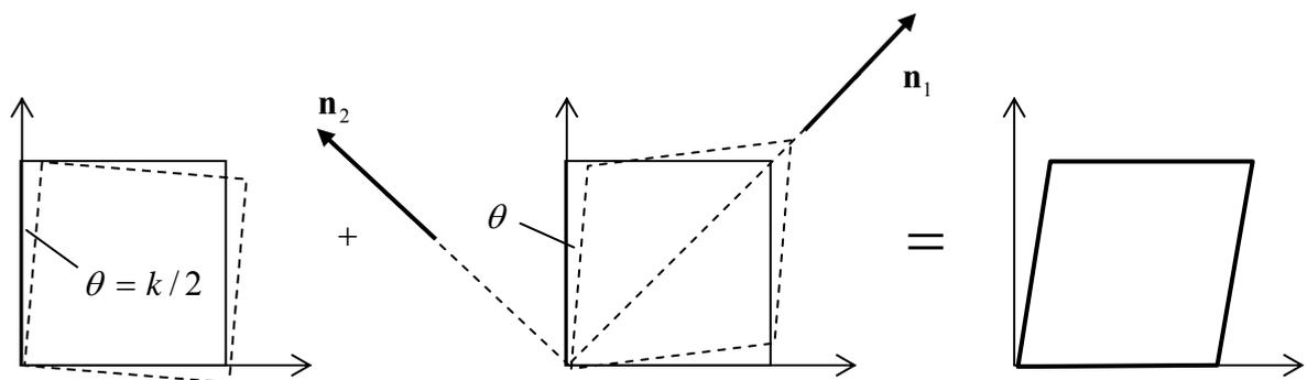
Figure 2.6.2: simple shear
