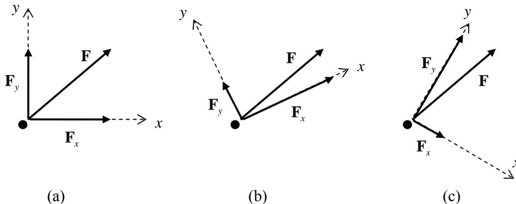
**Figure 2.2.1: A force  $\mathbf{F}$  decomposed into components  $\mathbf{F}_x$  and  $\mathbf{F}_y$  using three different coordinate systems**
