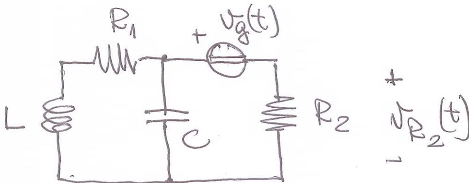
$$R_1 = 1\Omega; \quad R_2 = 1\Omega; \quad L = 1H; \quad C = 1F; \quad v_g(t) = \begin{cases} 1 & t < 0 \\ 0 & t \geq 0 \end{cases}$$
