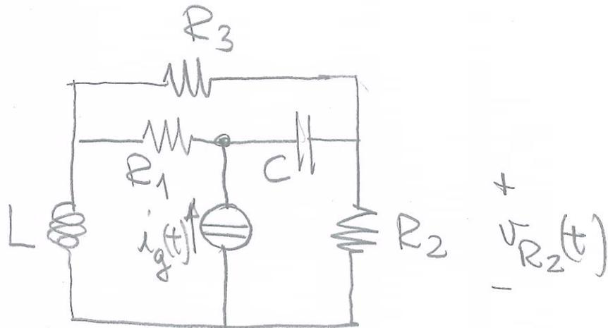
$$R_1 = 1\Omega; \quad R_2 = 1\Omega; \quad R_3 = 1\Omega; \quad L = 1H; \quad C = 1F;$$
