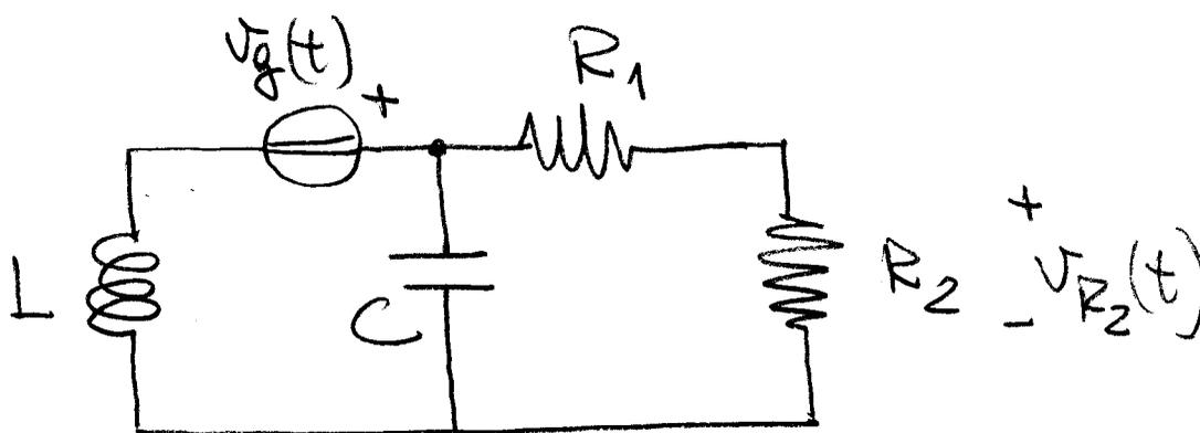
$$R_1 = 1\Omega; \quad R_2 = 1\Omega; \quad L = 1H; \quad C = 1F; \quad v_g(t) = \begin{cases} 1 & t < 0 \\ 0 & t \geq 0 \end{cases}$$
