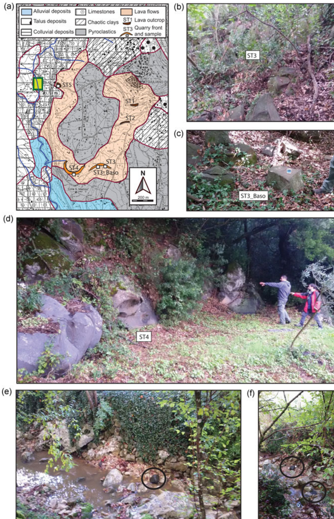
FIGURE 7 Field survey near the Giuliano di Roma village: (a) geological map of the investigated outcrops and stone quarry fronts; (b) quarry edge with detached rock blocks at site ST3; (c) reworked rock block from which sample ST3_Baso was taken; (d) quarry edge at site ST4; (e,f) evidence of semifinished volcanic blocks abandoned in an N-S flowing stream located west of the volcanic quarries (panel a for location) [Color figure can be viewed at wileyonlinelibrary.com ]
