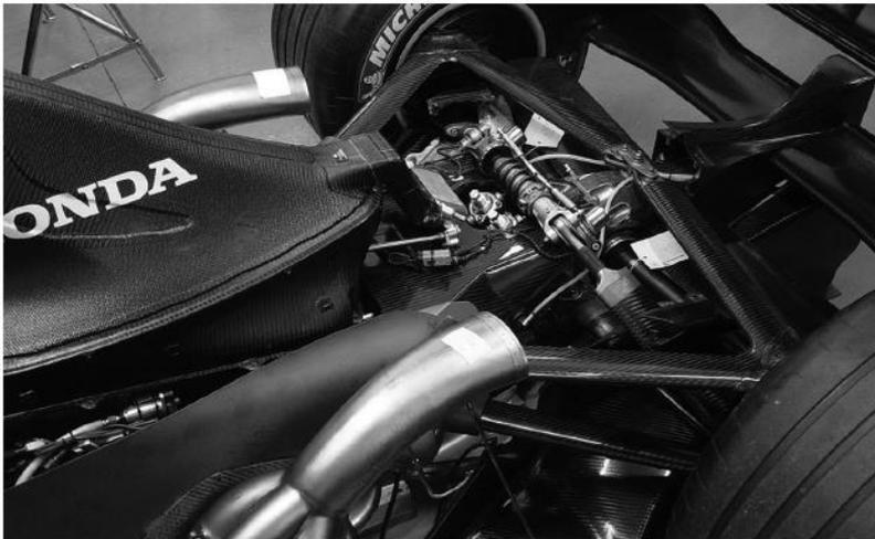
FIGURE 1.9 Carbon fiber-reinforced epoxy suspension and gear box in a Formula 1 race car. (Courtesy of Bar 1 Formula 1 Racing Team. With permission.)
