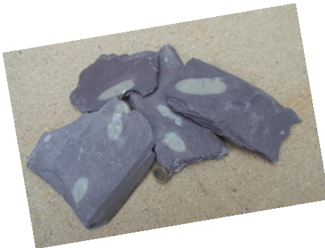
Ellipsoidal reduction spots in slate (elliptical in x-section) after strain and volume change, \Delta (Appalachians, USA).
