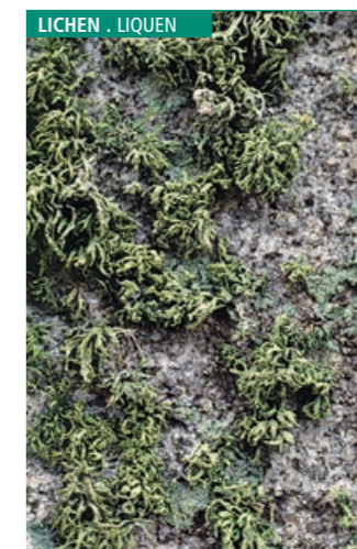
Folioid lichen ( Ramalina sp.) growing on a granite dimension stone.
