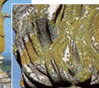
Folioid lichen ( Ramalina sp.) growing on a granite dimension stone.
