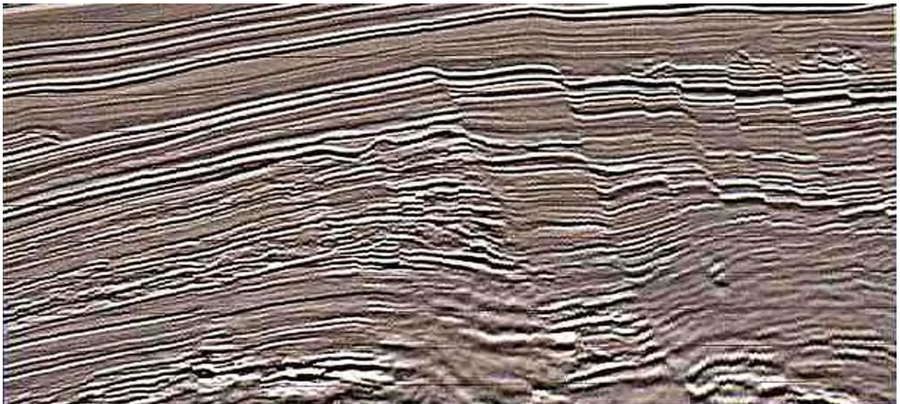
Fig. 95 - Seismic line showing a rotational, mainly planar domino set of extensional faults. Gulf of Mexico.
