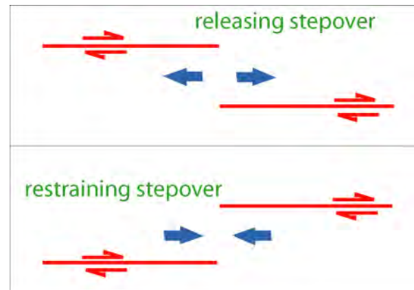
Fig. 120 - Strike slip segmentation and en-echelon stepover geometries may cause local shortening (restraining stepovers) or stretching (releasing stepovers). Stretching areas associated to releasing stepovers are called pull-apart basins, whereas the opposite restraining stepovers generate push-ups.
