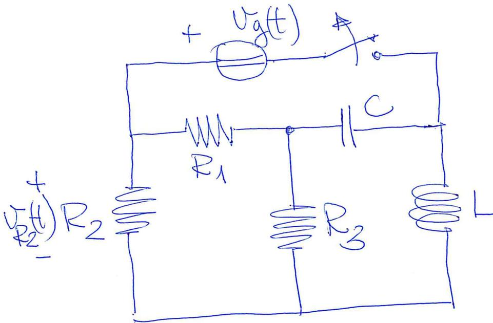
$$R_1 = 1\Omega; \quad R_2 = 1\Omega; \quad R_3 = 1\Omega; \quad L = 1H; \quad C = 1F; \quad v_g(t) = 1V$$
