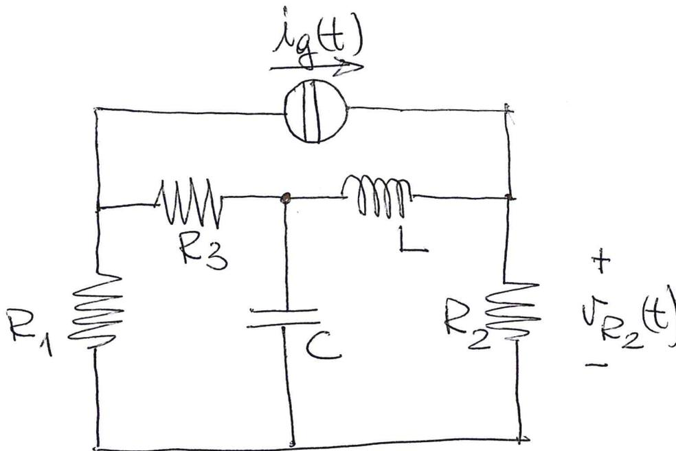
$$R_1 = 1\Omega; R_2 = 1\Omega; R_3 = 1\Omega; L = 1H; C = 1F; \quad i_g(t) = \begin{cases} 1 & t < 0 \\ 0 & t \geq 0 \end{cases}$$
