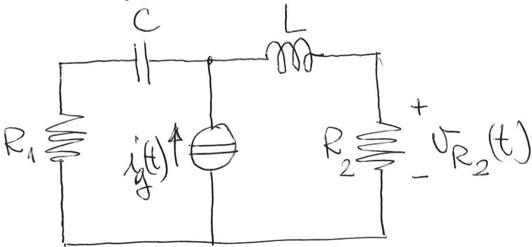
$$R_1 = 1\Omega; \quad R_2 = 1\Omega; \quad L = 1\text{H}; \quad C = 2\text{F}; \quad i_g(t) = \begin{cases} 1 & t < 0 \\ 0 & t \geq 0 \end{cases}$$
