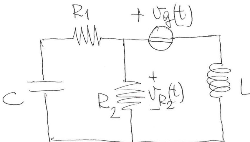
$$R_1 = 1\Omega; \quad R_2 = 1\Omega; \quad L = 1\text{H}; \quad C = 1\text{F}; \quad v_g(t) = \begin{cases} 1 & t < 0 \\ 0 & t \geq 0 \end{cases}$$
