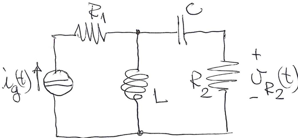
$$R_1 = 1\Omega; \quad R_2 = 1\Omega; \quad L = 1H; \quad C = 1F; \quad i_g(t) = \begin{cases} 1 & t < 0 \\ 0 & t \geq 0 \end{cases}$$
