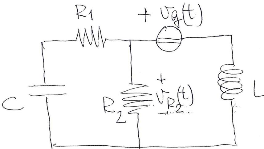
$$R_1 = 1\Omega; \quad R_2 = 1\Omega; \quad L = 1H; \quad C = 1F; \quad v_g(t) = \begin{cases} 1 & t < 0 \\ 0 & t \geq 0 \end{cases}$$
