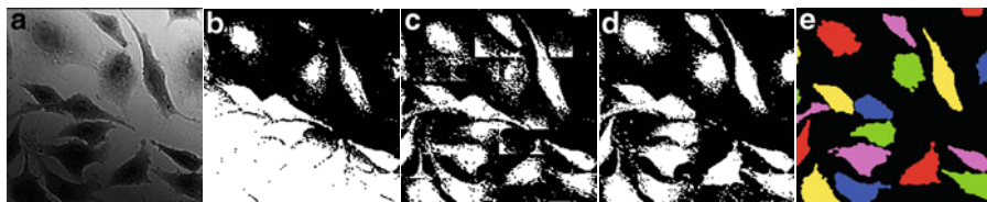
Fig. 1.26. Dynamic thresholding in microscopy [8]. The microscopy of a cell culture (a) was segmented using a global threshold (b), locally adaptive (c) and pixel-connected (d). According to morphological post-processing for noise reduction and a connected components analysis, the final segmentation is shown in (e)
