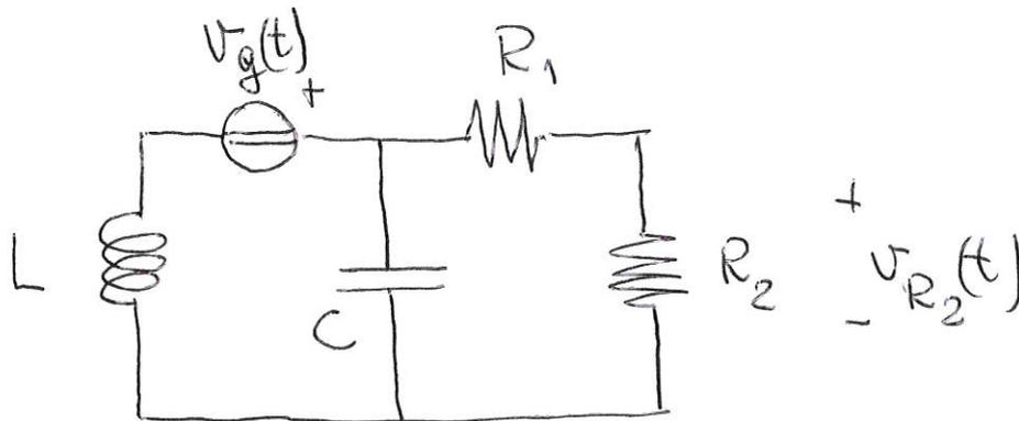
$$R_1 = 1\Omega; \quad R_2 = 1\Omega; \quad L = 1H; \quad C = 1F; \quad v_g(t) = \begin{cases} 1 & t < 0 \\ 0 & t \geq 0 \end{cases}$$
