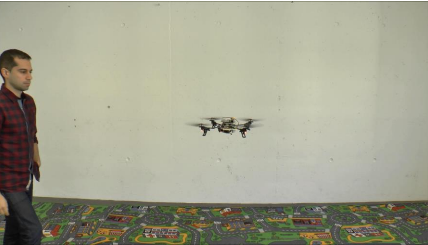
RMS error: 5 mm, height: 1.5 m – Down-looking camera
